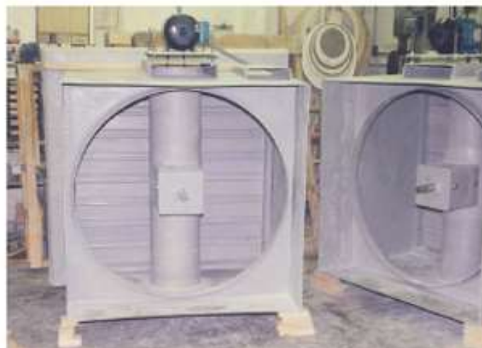
48 inch diameter belt drive wall fans with motor out of the air
