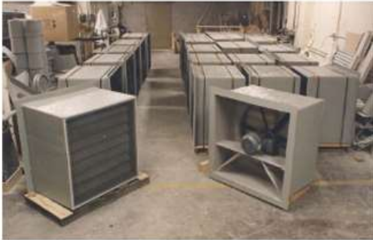
60 inch Diameter Direct Drive wall fans with intake air shutter
