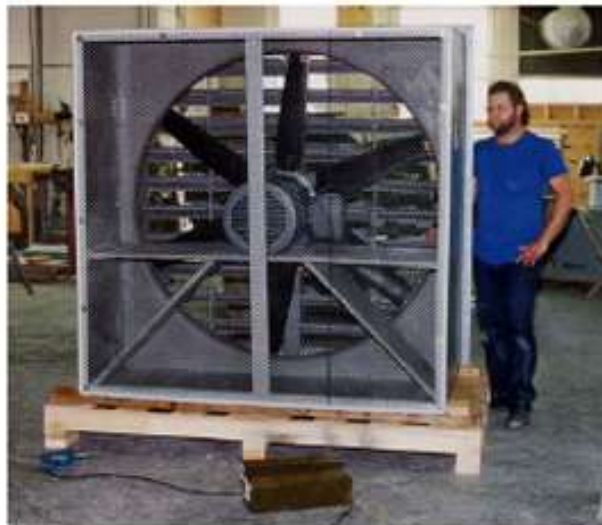
Production run of 36 inch diameter Wall Box Fans
