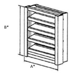
\*NOTE: Opening size is normally 1/4" larger than louver size. Structural support of louver in opening by others. Screen adds approximately 1/2" deep
