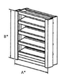
\*NOTE: Opening size is normally 1/4" larger than louver size. Structural support of louver in opening by others. Screen adds approximately 1/2 " deep
