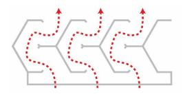
Warm air rises through the unit moving around the ventilator blades.
